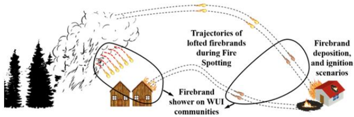
Schematic of the three main phases of the firebrand shower, i.e. (1) firebrand generation, (2) firebrand transport and (3) thermal exposure and spot fire ignition.
